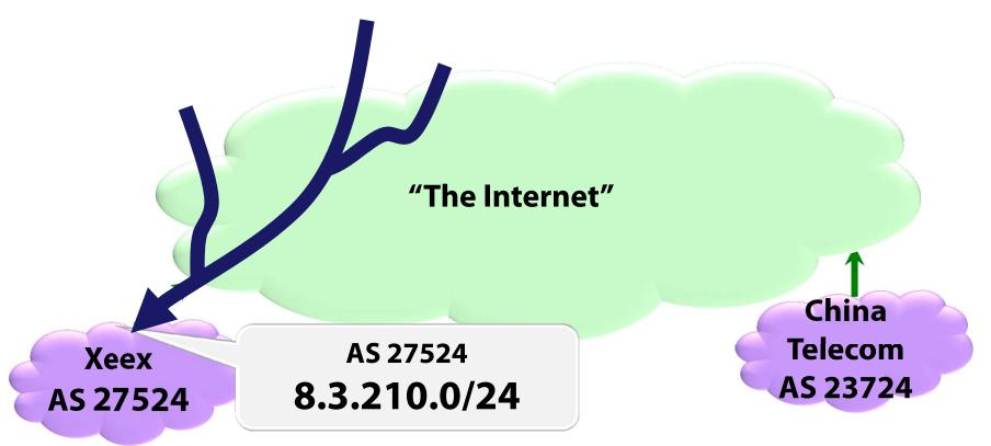
The internet is a graph. Each node is an AS (autonomous system), with an identifying AS Number.
