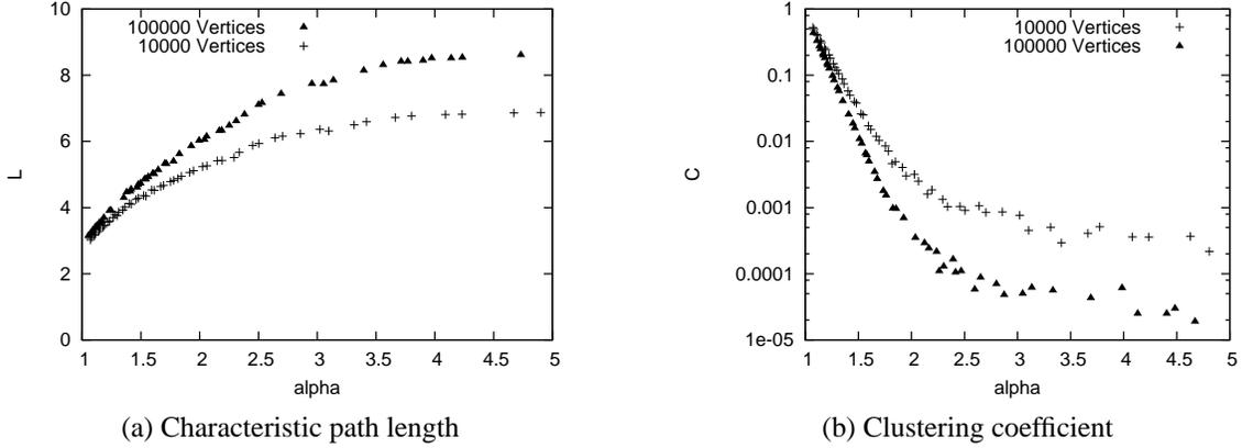
Figure 2: Power Law vertex degree distribution results in small-world behavior. Smaller power-law exponent (higher variability) results in shorter path length and stronger clustering.
