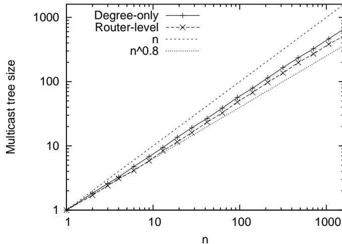
Figure 11: Comparison of the scaling behaviors of IP multicast using degree-only topology and real Internet topology.
