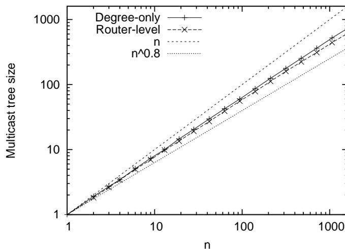
Figure 13: Comparison of the scaling behaviors of end-system multicast using degree-only topology and real Internet topology.
