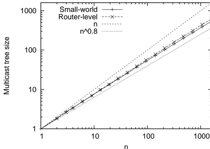
Figure 14: Comparison of the scaling behaviors of end-system multicast using small-world topology and real Internet topology.
