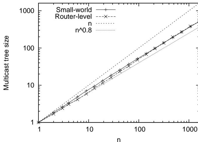
Figure 12: Comparison of the scaling behaviors of IP multicast using small-world topology and real Internet topology.
