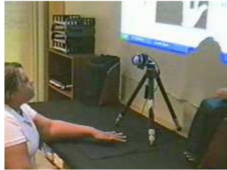
Figure 10. MUSIC MAKER: A camera-based music making tool for rehabilitation. The user obtains visual and auditory feedback based on the analysis the motion pattern of her hand (Fig. courtesy of Gorman et al. [15]).
