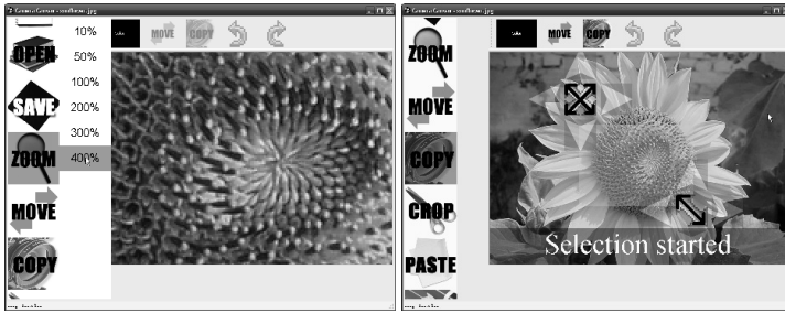
Fig. 7 Image-editing tool CAMERA CANVAS. Left: A Camera Mouse user selected the 400%-zoom option while working with a sunflower picture. Right: To crop and copy an image region, the user must select the position of the upper left corner of the region and the size (i.e., position of lower right corner) of the region by moving the mouse pointer onto one of the arrows.
