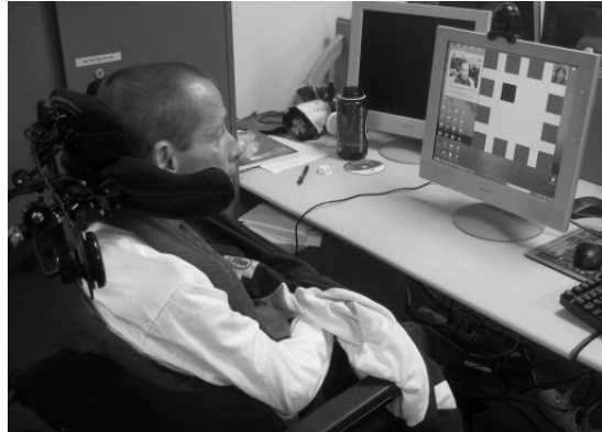
Fig. 1 A CAMERA MOUSE user who is quadriplegic due to cerebral palsy. The user moves the mouse pointer to the different regions on the screen by slightly moving his head. In the left upper region of the screen, a window with the Camera Mouse interface can be seen that contains the currently processed video frame showing the user’s face. The camera that captured this frame is attached to the top of the monitor (black).
