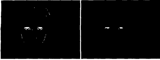
Figure 2: Thresholded difference image prior to erosion (left), and same image after erosion (right). Erosion removes noise caused by insignificant motion in the scene.
