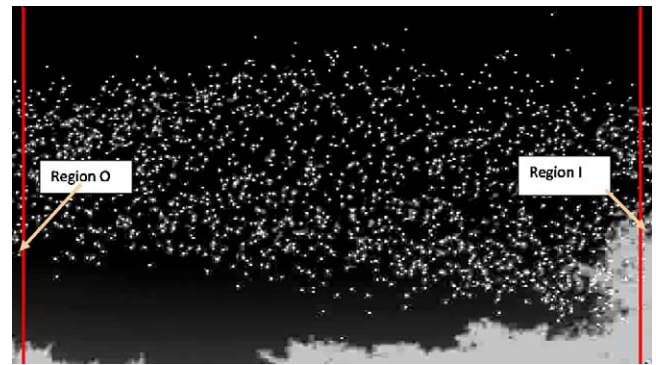
Fig. 3. Bats enter the frame on the right (region I). Our method counts the bats leaving the frame on the left (region O). The width of the regions is 1/72 of the width of the frame.
