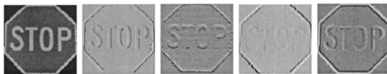
Figure 13. A stop sign and its partial derivatives with respect to x , y , \theta , and s = s_x = s_y .
