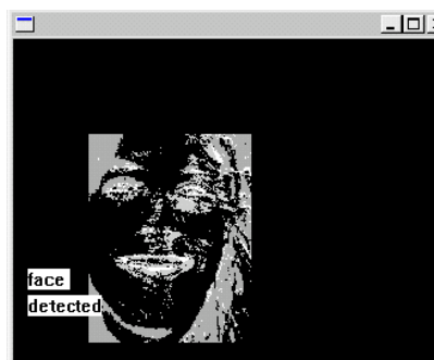
Figure 2: Composite image: Most likely eye pixels are shown in white. Pixels that are either part of a strong horizontal edge, or belong to a dark region are shown in gray. Pixels that do not fulfill either criterion are shown in black.
