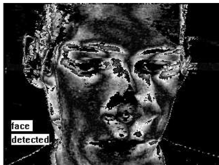
Figure 5: A skin-tone motion image. Bright pixels indicate significant temporal changes in skin tone, black pixels indicate no change.
