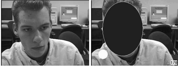
Figure 6: The face in the left image is detected and modeled by the ellipse shown in the right image.
