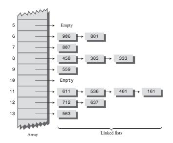
FIGURE 11.10 Example of separate chaining.
