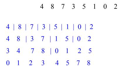
(B) What is the O(...N....) time complexity of just the merge operation of the algorithm? O( N )
