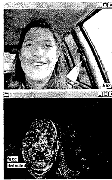
Figure 1: An original image and its skin-tone motion. Bright pixels indicate significant temporal changes in skin tone, black pixels indicate no change.
