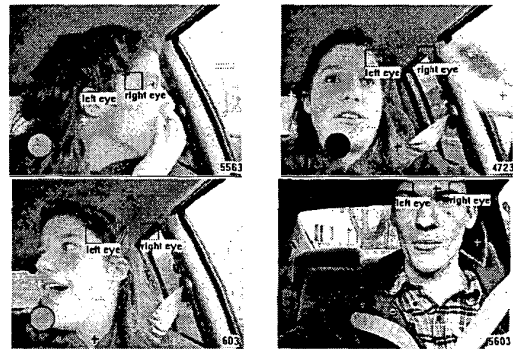
Figure 7: Incorrect localization of eyes due to occlusion, fast motion, and incorrect face localization.
