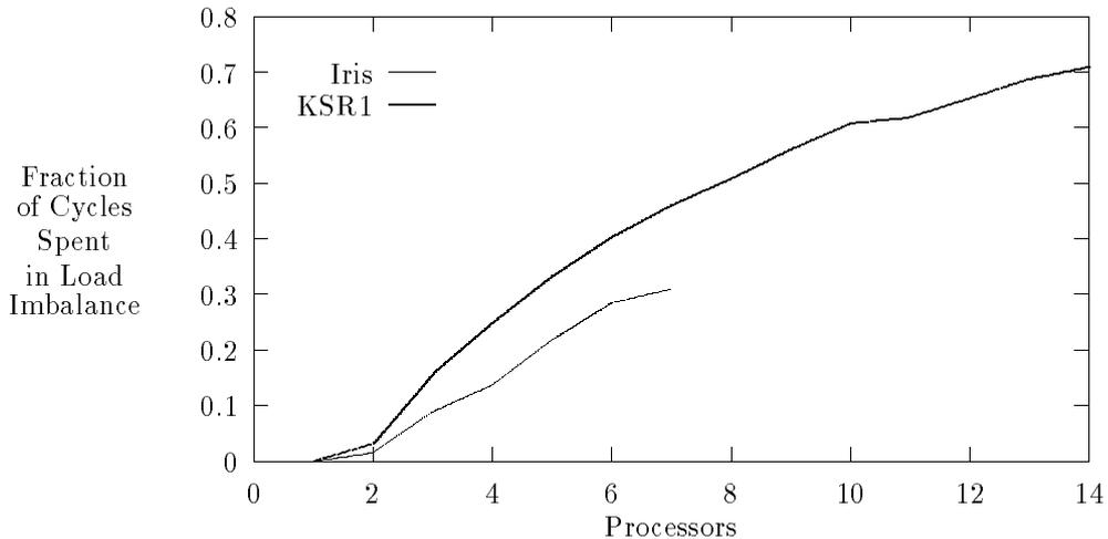
Figure 3: Increasing Load Imbalance in Loop Parallelism
