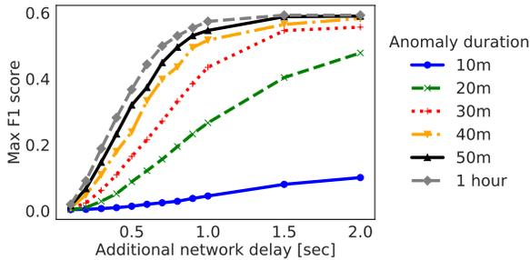
**Fig. 4**— Effect of anomaly duration and severity on WMF’s maximum F1 score.
