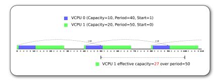
• Over-capacity exploit without proper splitting of replenishments
