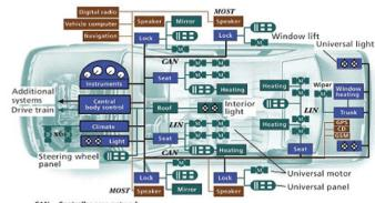
CAN Controller area network GPS Global Positioning System GSM Global System for Mobile Communications LIN Local interconnect network MOST Media-oriented systems transport
