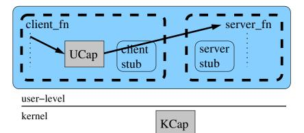
Switching between the two isolation levels requires changing UCap, KCap, and protection domains
