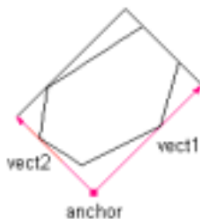
Figure 4-3 Minimal Area Bounding Rectangle
