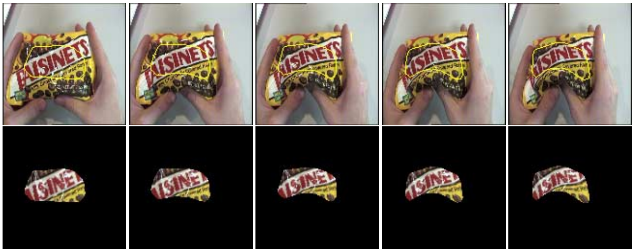
Figure 4: On-line tracking a deforming plastic bag filled with candy using difference decomposition. This figure shows every twentieth frame in the tracking sequence. For visualization purposes, an outline of the active blob is shown overlaid on the original input images. Marquardt-Levenberg minimization averaged 0.9 frames/sec, while the difference decomposition averaged 8.4 frames/sec. Results for the difference decomposition are shown below each input image. Marquardt-Levenberg was not able to track the object completely through this sequence.
