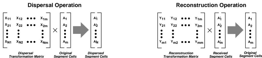
Figure 3: The Dispersal and Reconstruction operations of IDA.
