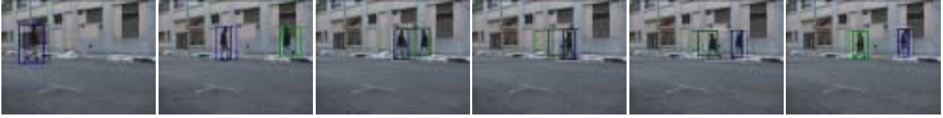
Figure 8: Tracking results, non-linear trajectories. Bodies are tracked, but prediction is less accurate because of sudden change in direction during occlusion.
