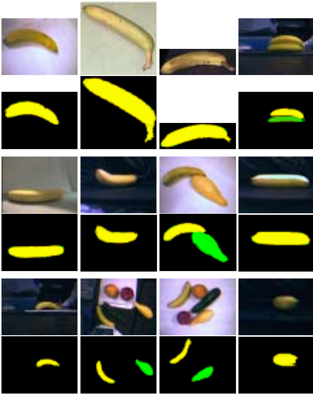
Figure 3: Image segmentation example: color images of bananas in various positions with varying illumination. The resulting model-based region groupings are shown below each color input image. If an image contained more than one detected shape, the shape that the system recognized as most “banana like” in each image is labeled in light gray. Note that the most similar shapes are other bent bananas of similar aspect ratio.
