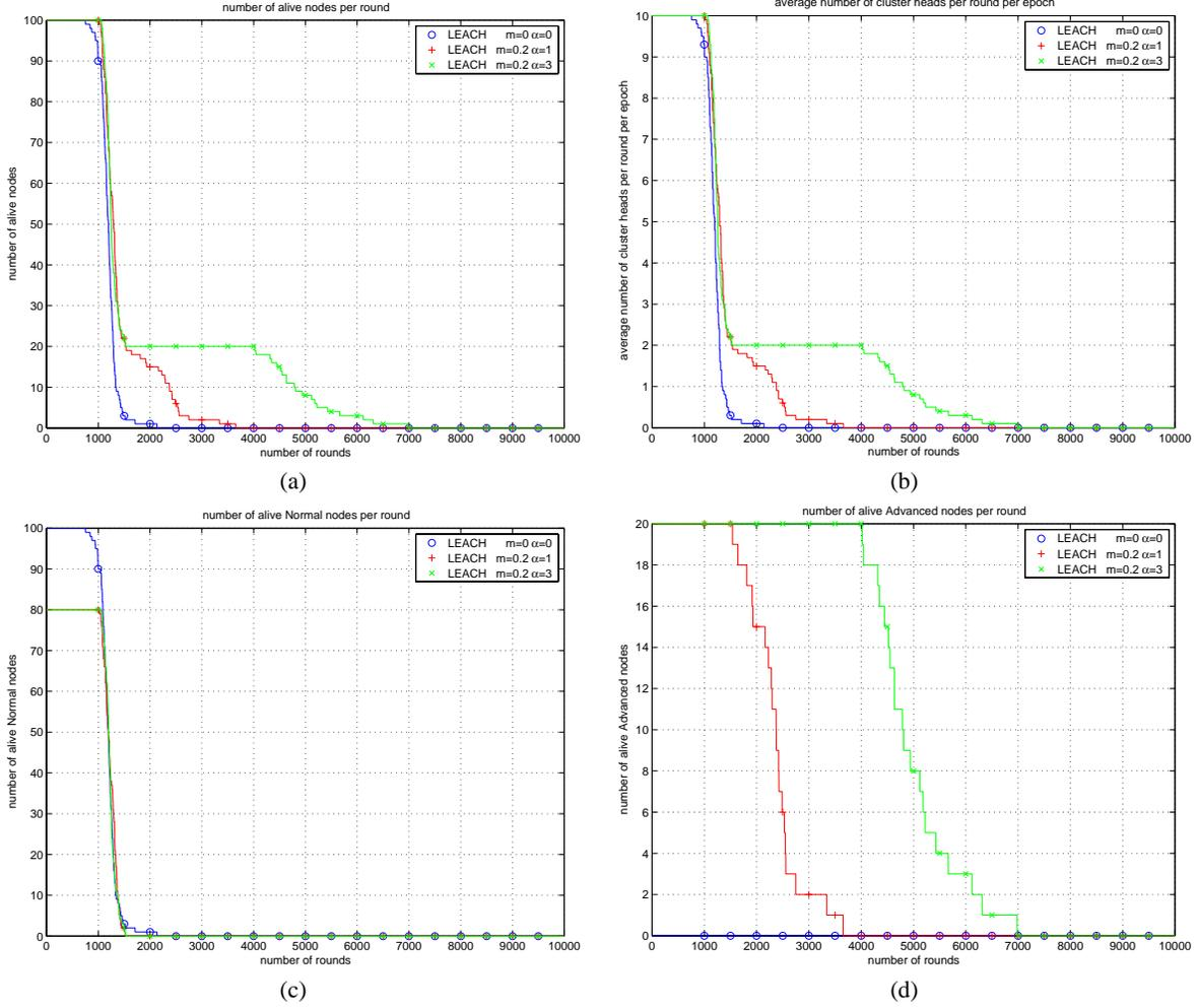
**Figure 7: LEACH behavior in the presence of heterogeneity with  $m = 0.2$  and  $\alpha = 3$ : (a) Alive nodes per round; (b) Average number of cluster heads per round per epoch; (c) Normal nodes per round; (d) Advanced nodes per round**
