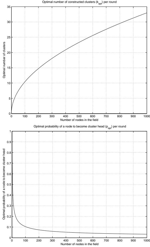
**Figure 2: (top) Optimal number of clusters; and (bottom) Optimal probability of a node to become a cluster head, as a function of number of nodes in a  $100m \times 100m$  field where the sink is located in the center.**
