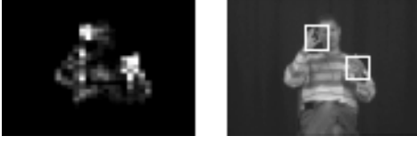
Figure 2: On the left is the motion residue of two frames in Figure 1. On the right is the located hands in current frame
