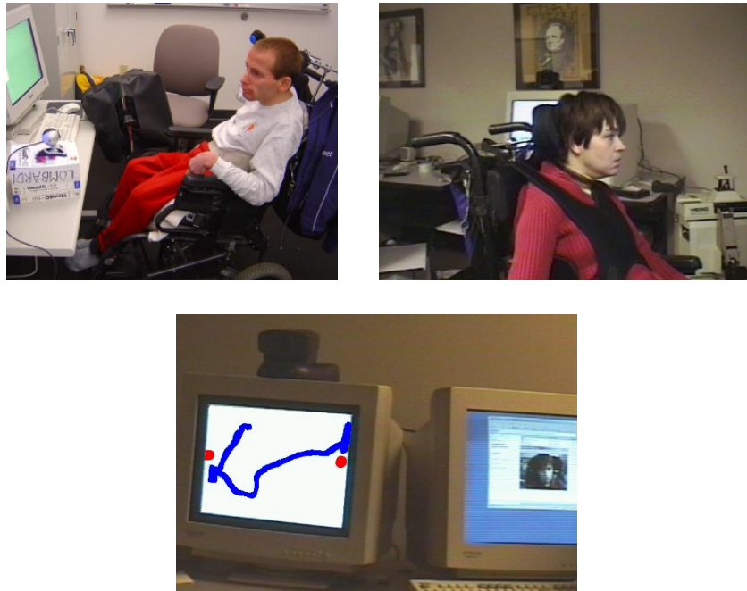
Figure 7: Subject 1 (top left image) and subject 2 (top right image) are using the Camera Mouse as a mouse-pointer substitution interface. Subject 2’s attempt to draw a vertical line is shown in blue on the left monitor in the bottom image. The subject was instructed to draw a straight line between the two red regions. She failed to reach both regions. During the drawing, the subject’s face and the tracking results of the Camera Mouse were observed on the monitor to the right. It was verified that the Camera Mouse was functioning correctly and that the drawn pattern corresponded to the user’s head motion.
