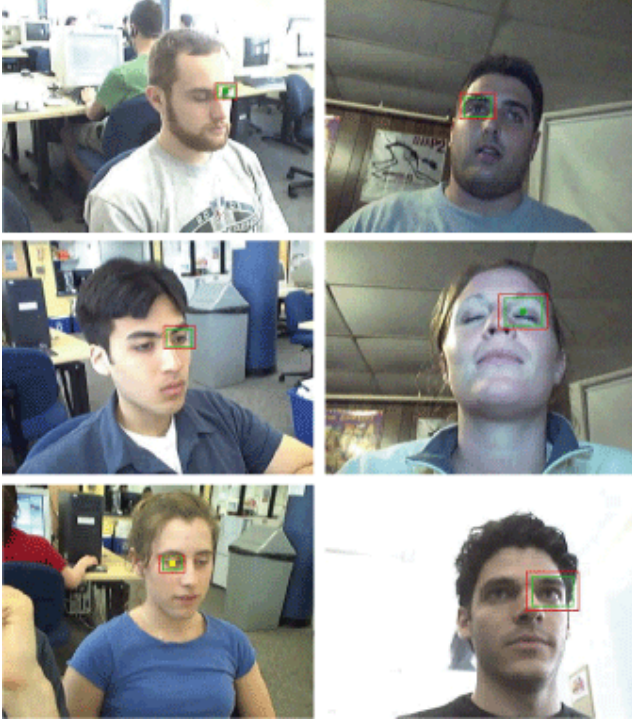
Figure 9: Sample frames from sessions testing alternate positions of the camera. The system still works accurately with the camera placed well below the user’s face, as well as with the camera rotated as much as about 45 degrees.
