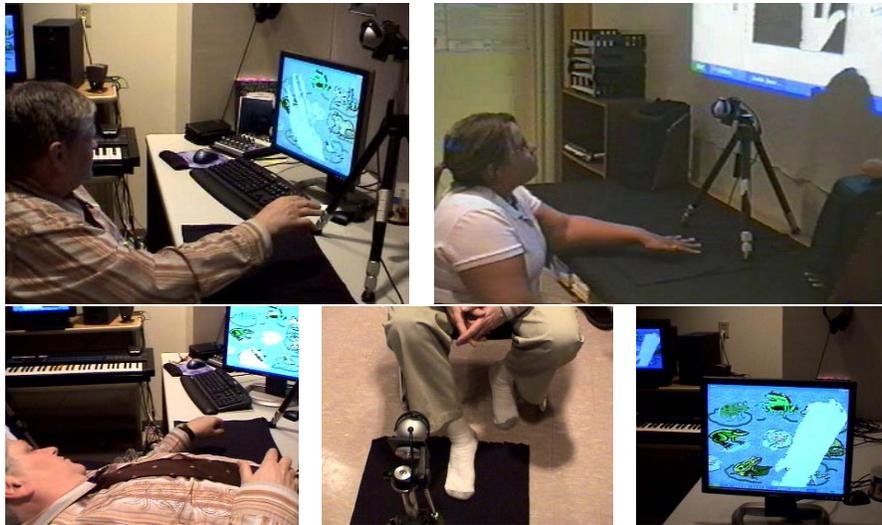
**Fig. 1.** Music Maker in use. It observes the movements of the users’ hands (top row and bottom left) or foot (bottom middle and right) with a downward-facing camera, interprets them, and provides auditory and visual feedback to the user. Visual feedback is provided with a monitor display (top left and bottom row) and a screen display (top right).
