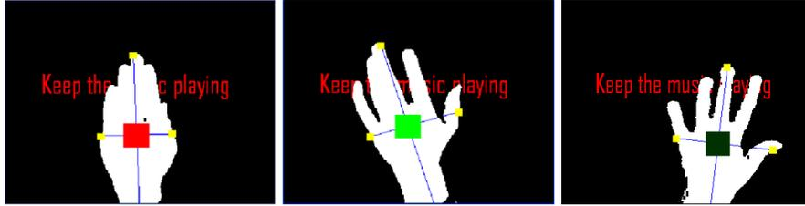
**Fig. 4.** Left: Stationary hand shown in a red centroid. Middle: Fast moving hand. The speed is indicated by green centroid. Right: Slowly moving hand. The speed is indicated by a dark green centroid.
