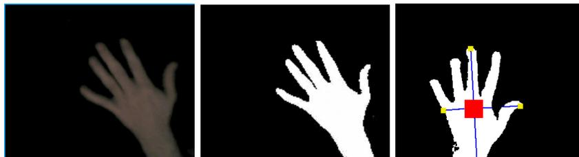
**Fig. 3.** Left: Camera view of a subject’s hand. Middle: Filtered binary image of detected hand. Right: Binary hand image with centroid in red, axes of least and most inertia in blue, intersection points in yellow.
