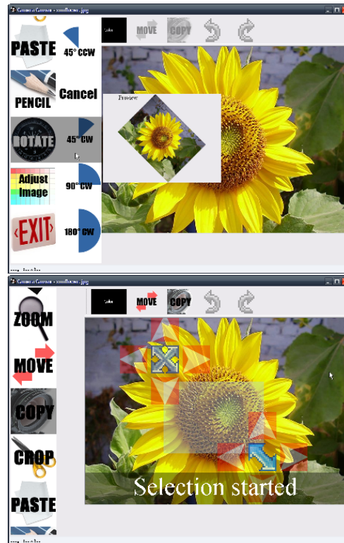
Fig. 4 The CAMERA CANVAS image editing tool. The user scrolls through the menu bar on the left by moving the mouse pointer up or down. To select a task, the pointer must dwell on the gray icon in the center of the bar. Top: Image rotation. The user selected to rotate the image 45 degrees counterclockwise (CW) on the second menu bar. Bottom: Copy Interface. The user selected the portion of the image to copy represented as a translucent blue rectangle. To change the position and size of the rectangle, the user moves the upper left and lower right corner of the rectangle, respectively. The movement is initiated by placing the mouse pointer onto one of the white-red arrows (Figure courtesy of Kim et al (2008)).
