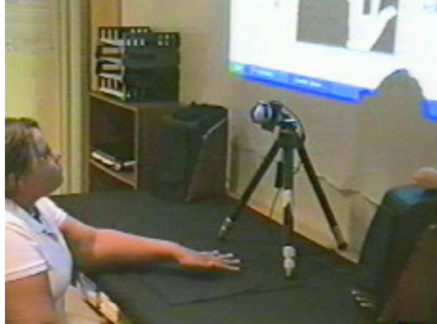
Fig. 10 MUSIC MAKER: A camera-based music making tool for rehabilitation. The user obtains visual and auditory feedback based on the analysis the motion pattern of her hand (Figure courtesy of Gorman et al (2005)).
