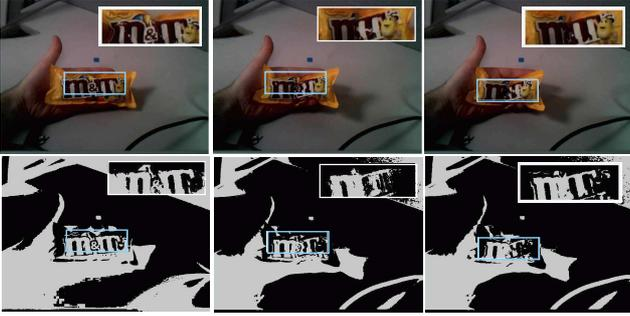
Figure 6. Tracked deformations of a candy wrapper (explanation in Fig. 4). The tracker correctly detects the increasing level of folding.
