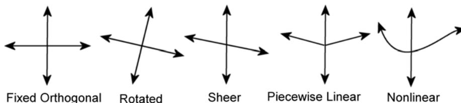
**Fig. 3.** Adaptive pointer-movement functions for mouse-replacement systems.
