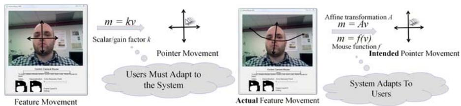
**Fig. 2.** Conceptual design of pointer movement functions. In a traditional mouse-replacement system, the mouse control function maps the facial feature motion linearly to the mouse pointer motion on the screen (left). In an adaptive system, the user’s head motion is transformed into the intended mouse motion with a nonlinear function.
