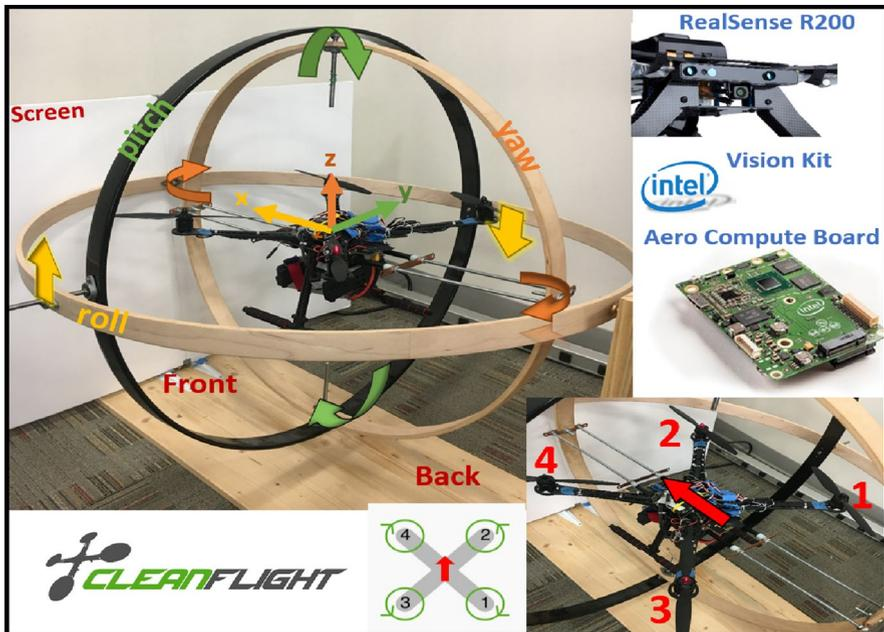
Fig. 7 BirdCage testbed for real-world experiments. The quadcopter motor configuration is enumerated at the bottom-right
