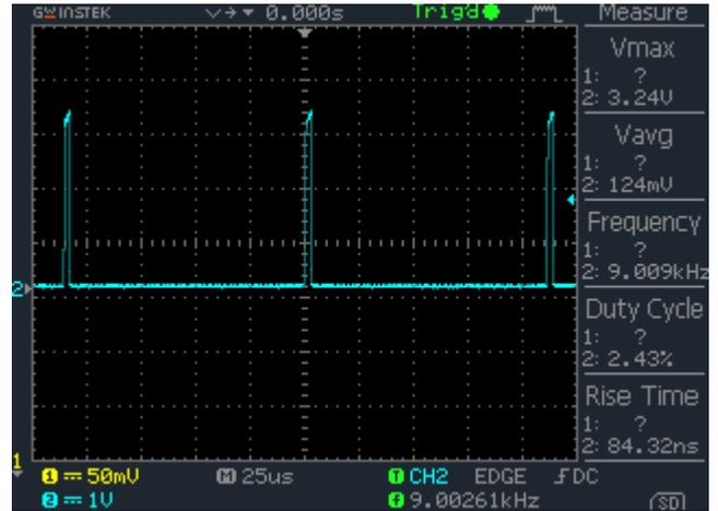
Fig. 11: Target 10kHz Pulse on Qduino (Actually 9.009kHz)
