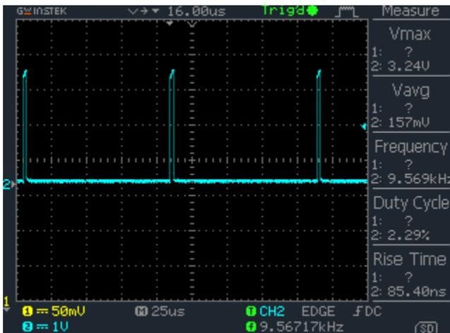
Fig. 12: Target 10kHz Pulse on QduinoMC (Actually 9.569kHz)
