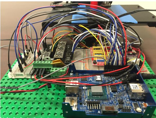
Fig. 14: MinnowMax-based Controller for the Printbot
