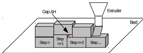
Fig. 3: Structural Deficiency due to Unstable Pulse Train
