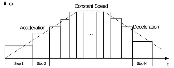
Fig. 2: An Example Speed Ramp for a Stepper Motor
