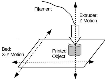
Fig. 1: A Conceptual View of a 3D Printer
