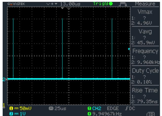
Fig. 13: 10kHz Pulse on the Printboard (without a webserver)
