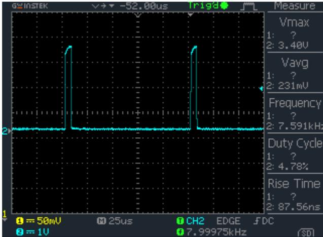
Fig. 10: Target 10kHz Pulse on Yocto Linux (Actually 7.591kHz)
