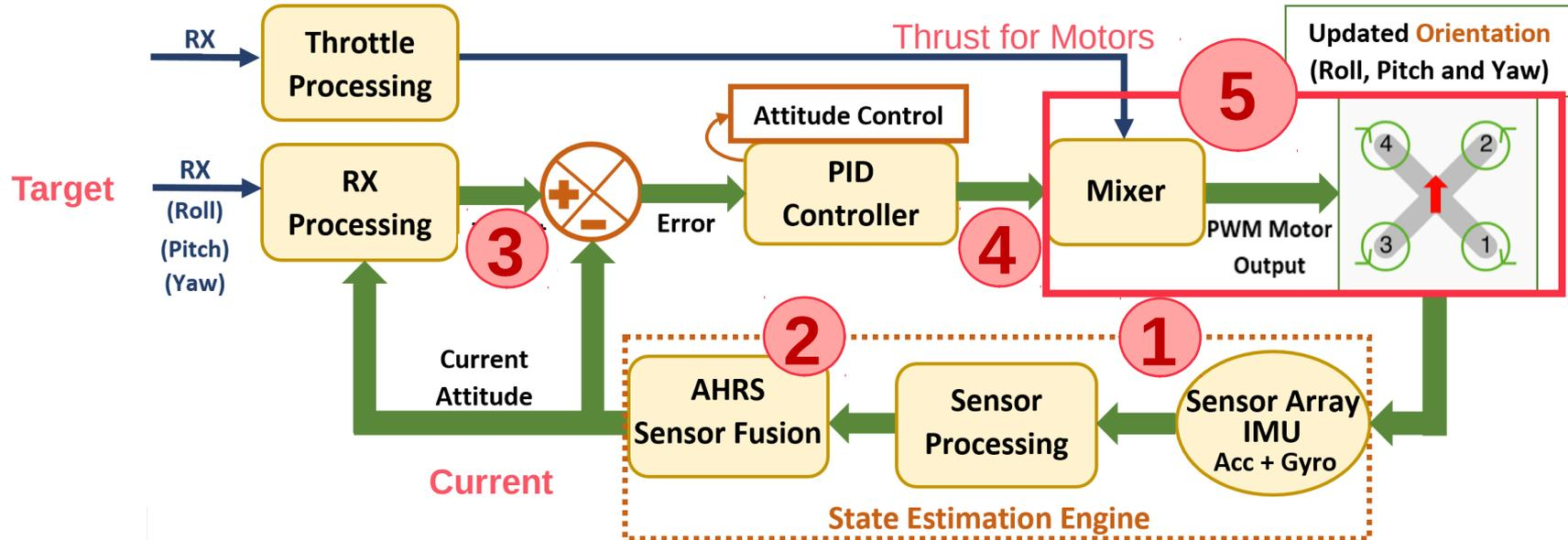
Low-level attitude stabilization: **classical linear feedback control loop**
