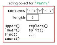
• Because a method is inside the object, it is able to access the object's attributes.
