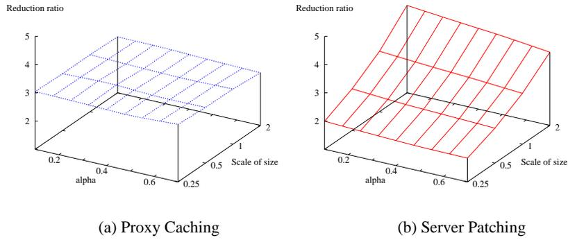
Figure 1.8. Server bandwidth reduction ratios of proxy caching and server patching schemes when size distribution parameters change. Larger sizes favorites server patching.
