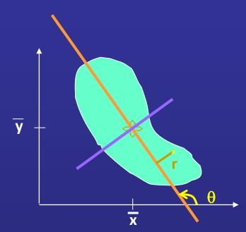
Axis of least inertia = Direction of elongation min E = min  $\Sigma\Sigma$  r<sup>2</sup>
