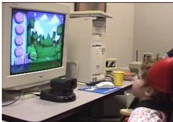
Figure 3: The Camera Mouse user playing with educational software. The video camera is placed underneath the user computer's monitor.
