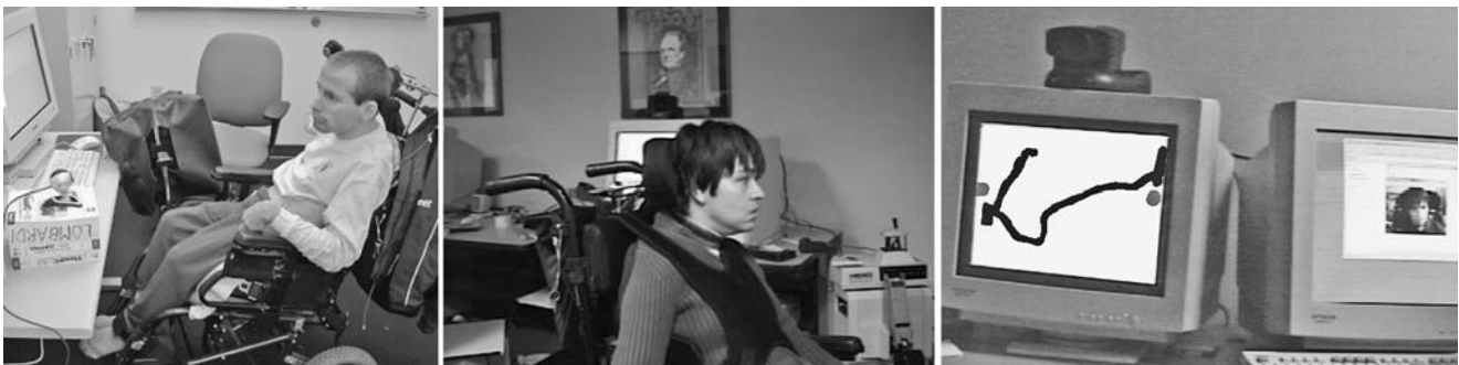
Fig. 7 Subject 1 ( left image ) and subject 2 ( middle image ) are using the Camera Mouse as a mouse-pointer substitution interface. Subject 2s attempt to draw a vertical line is shown in blue on the left monitor in the right image . The subject was instructed to draw a straight line between the two red regions. She failed to reach both
