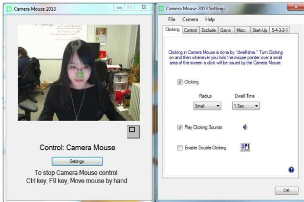
**Figure 1. The interface and configuration of Camera Mouse. The green box shows the feature tracked.**
