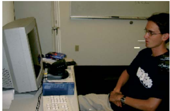
Fig. 13. A user accessing the computer with EYEBROWCLICKER. The camera is placed in front of the monitor but below the screen
