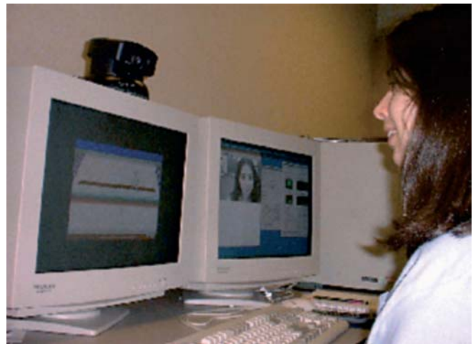
Fig. 12. BLINKLINK in use: the video camera is placed on top of the left monitor, which displays the application software. The right computer monitor (not required) is used to check the status of the system. A user plays an arcade game based on scanning software where the objective is to throw a baseball at plates on a shelf. A long blink causes a ball to be thrown. The user must time the blink so that it coincides with the highlighting of a plate
