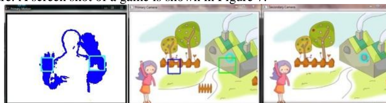
Figure 7. Hidden Paintings : The interface contains windows that display two versions of a picture* and tracking results. The detected hand locations (cyan) are shown overlaid onto the binary version of the motion energy image. The tracked locations of the left and right hands are mapped to corresponding positions in the original version of the picture (blue and green rectangle). The goal of the user is to move the rectangles onto the objects that do not appear in the other version of the picture, here the fence and the red apple. (* The original picture was obtained from Google Image Search and manipulated with image editing software to create a version with “hidden” objects.)
