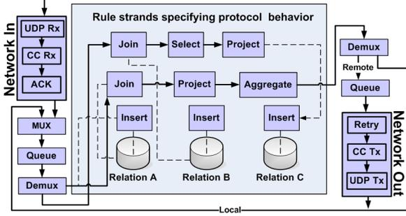
Figure 2: P2's Dataflow Architecture
