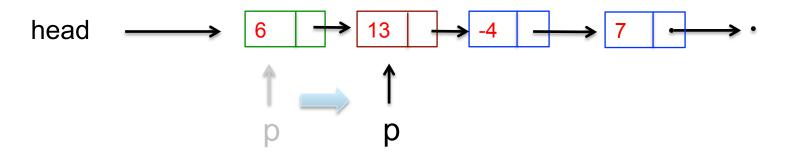
We can move down the list by assigning a point p to point to head,
