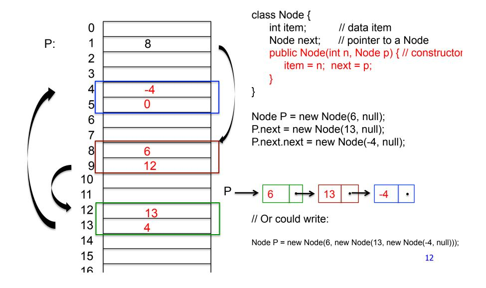
Be **SURE** that you understand the different uses of a variable in an assignment statement:
