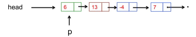
We can move down the list by assigning a pointer p to point to head,
