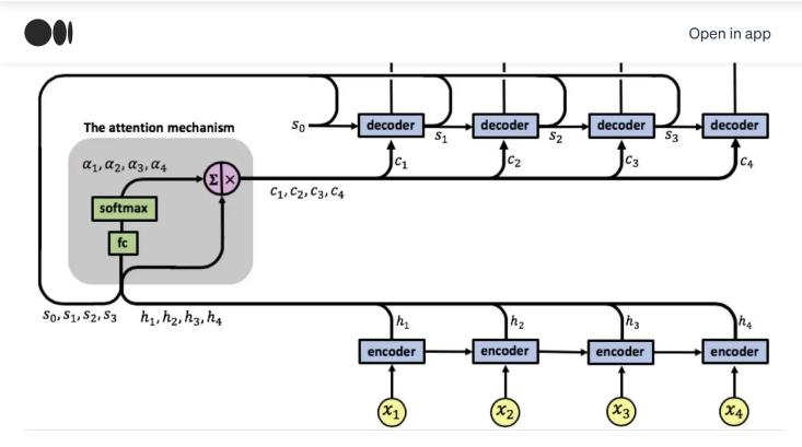
Our attention model has a single layer RNN encoder, again with 4-time steps. We denote the encoder's input vectors by x1, x2, x3, x4 and the output vectors by h1, h2, h3, h4.
