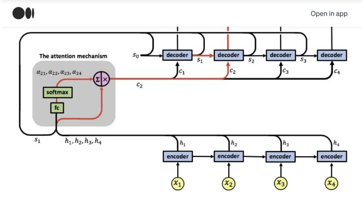
At the next time step the attention mechanism has an input sequence [s2, h1], [s2, h2], [s2, h3], [s2, h4].
