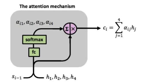
At time step i, the mechanism has h1,h2,h3,h4 and si-1 as inputs, it uses the fc neural network and the softmax function to compute the attention weights ai1, ai2, ai3, ai4, these are then used in the computation of the context vector ci.
