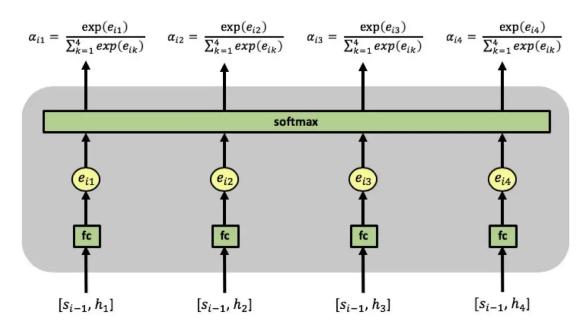
Computation of attention weights at time step i, notice how this needs to be computed separately on every time step since the computation at time step i involves si-1, the decoder's state form time step i-1
