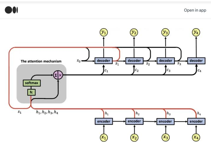
It computes a second set of attention weights α21, α22, α23, α24 enabling the computation of the first context vector c2. The decoder uses [s1,c2] and computes the second RNN output y2.
