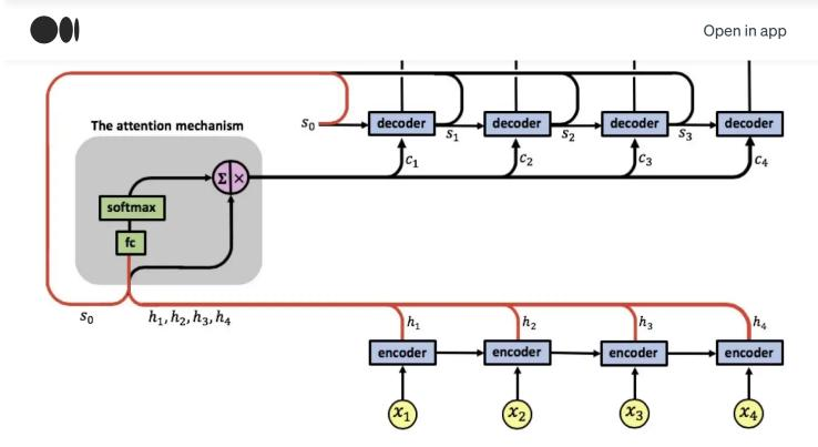
The attention mechanism computes the first set of attention weights  $\alpha 11$ ,  $\alpha 12$ ,  $\alpha 13$ ,  $\alpha 14$  enabling the computation of the first context vector c1. The decoder now uses [s0,c1] and computes the first RNN output y1
