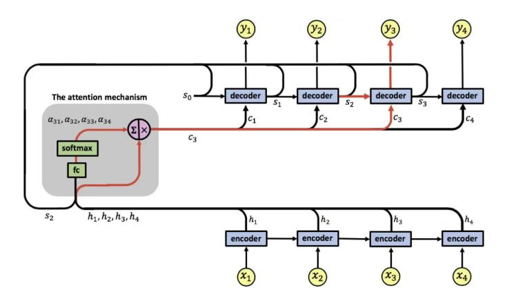
At the next time step the attention mechanism has an input sequence [s3, h1], [s3, h2], [s3, h3], [s3, h4].
