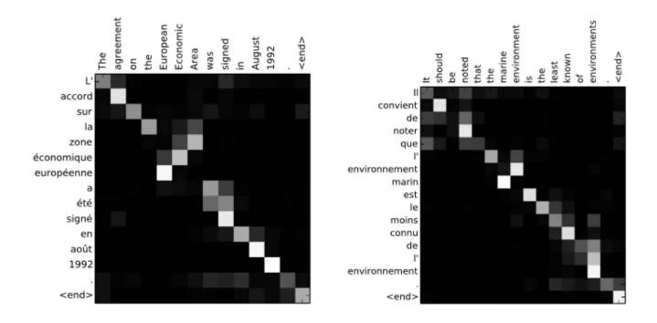
We see how the attention mechanism allows the RNN to focus on a small part of the input sentence when outputting the translation. Notice how the larger attention parameters (given by the white pixels) connect corresponding parts of the English and French sentences enabling the network in [1] to achieve state of the art results.
