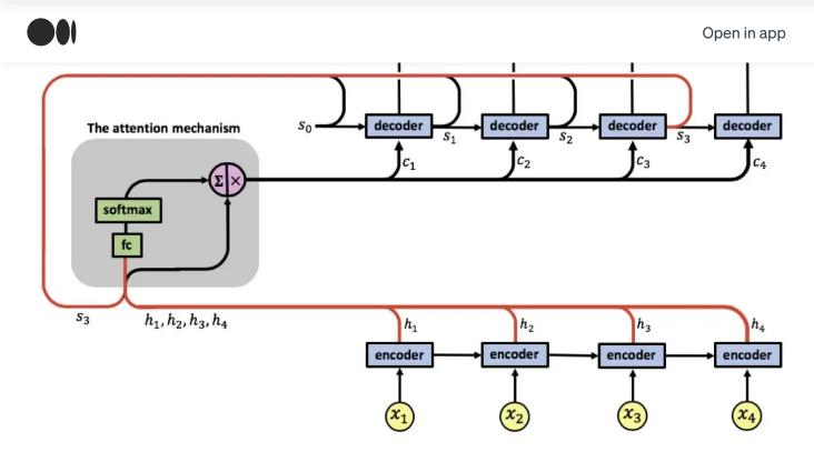
It computes a fourth set of attention weights α41, α42, α43, α44 enabling the computation of the fourth context vector c4. The decoder uses [s3,c4] and computes the final output y4.
