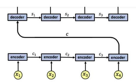
An RNN encoder-decoder architecture, we take an architecture with 4 time steps for simplicity
