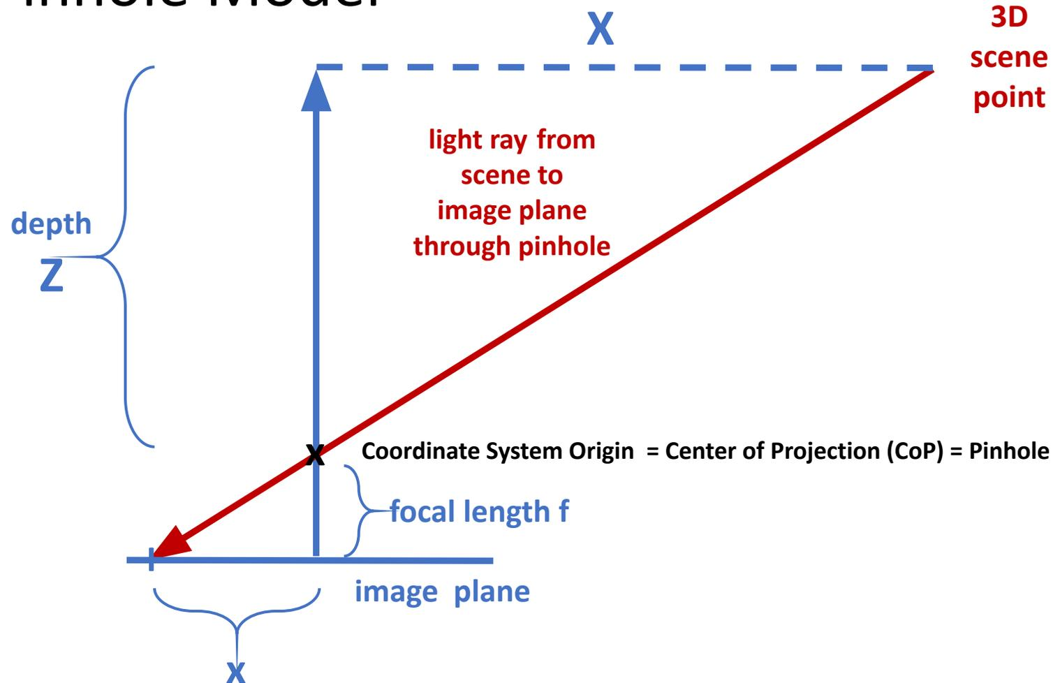
We can relate the scene and image plane coordinates  $X$  and  $x$  using a perspective projection equation.
