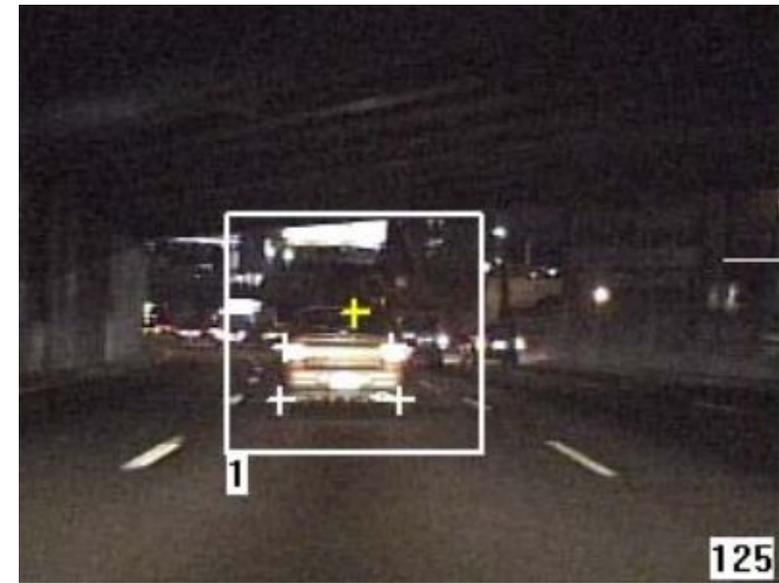
Distance in meters:  $Z = c_{\text{horiz}} f W / w = (22 \text{ pix/mm})(50 \text{ mm})(1.77 \text{ m}) / (100 \text{ pix})$
