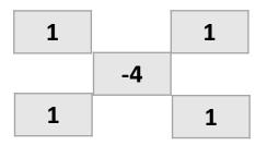
Accurate approximation of the Laplacian (linear combination of above):
