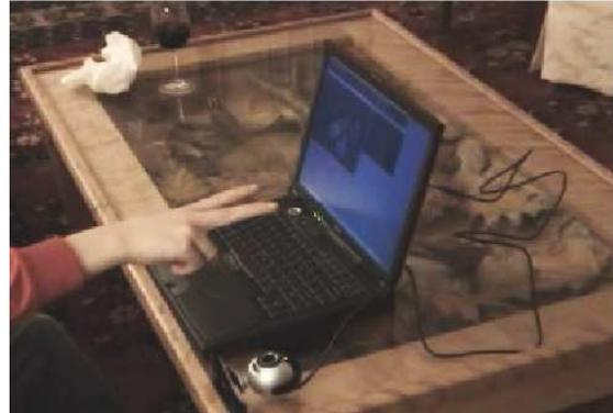
Fig. 1. The *Finger Counter*. The webcam (on the table) points upward at the hand.
