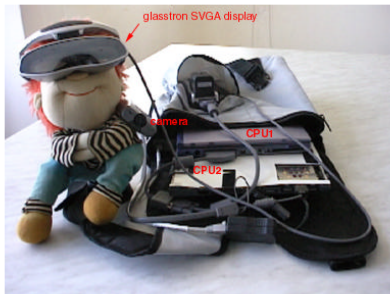
Figure 15. Wearable Cinema setup, showing the backpack, the two CPUs, the camera, and the lightweight color SVGA glasstron display.
