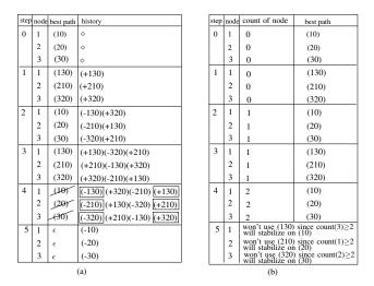
Fig. 3. (a) A possible trace of SPVP for the system shown in Figure 1; (b) A possible trace of the Cobb and Musunuri algorithm for the system shown in Figure 1 assuming threshold value for *count* is 2. All nodes stabilize on their lowest preferred paths.
