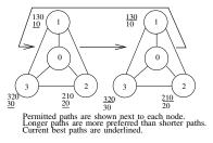
Fig. 1. An example of a divergence. Due to the cyclic conflict, this group of nodes cannot reach a stable state and keep oscillating between the shown states.
