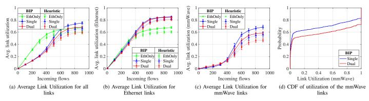
Figure 7: Average Link Utilization as a function of incoming flows for *EthOnly*, *Single* and *Dual* networks, and the CDF of mmWave link utilization
