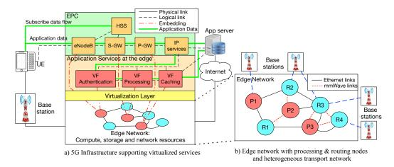
Figure 1: Function virtualization for 5G mobile network
